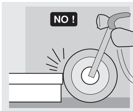
Avoid obstacles that could damage the vehicle or make you lose control. Avoid riding in the slipstream created by preceding vehicles in order to increase your speed.
