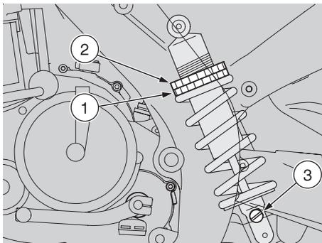
According to the conditions of use of the vehicle, it is possible to adjust the hydraulic braking with extended shock absorber by adjusting the screw (3); for the adjustment, keep to the following indications:
