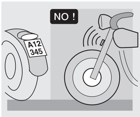
Never change the position, inclination or colour of: number plate, direction indicators, lights and horns.
