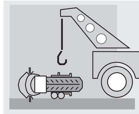
If the vehicle has been involved in an accident, make sure that no damage has occurred to the control levers, pipes, wires, braking system and vital parts.
